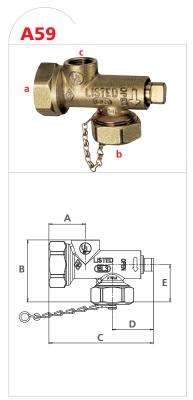
► For installing the last sprinkler head on system branch lines, controls water flow for flushing or testing of the system.
