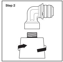
**Step 2.** Ensure O-ring is properly fitted beneath threads on neck of installation cup. Screw Installation Cup into sprinkler fitting ensuring top of installation cup is flush against face of sprinkler fitting.
