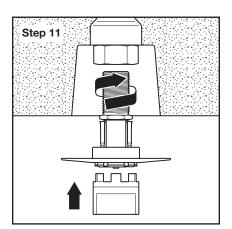
**Step 11.** Engage Sprinkler by W-Type 25 Wrench (Figure 2). Hand-tighten (19 Nm [14 ft.- lbs.] Maximum) assembly into Adapter. Ensure Escutcheon is flush against ceiling mounting surface and Sprinkler is oriented as intended (refer to Figures 1 and 2 for orientation details).
