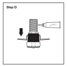
**Step D.** Assemble Escutcheon onto sprinkler body. Ensure Escutcheon is flush against sprinkler body mating surface. Apply sealant to external threads of thread extension.
