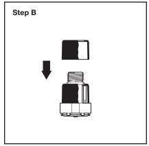
**Step B.** Assemble Dust Cap onto Sprinkler. Ensure Dust Cap is flush against sprinkler body mating surface.
