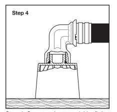
**Step 4.** Connect pipe to sprinkler fitting per manufacturer's recommendations.
