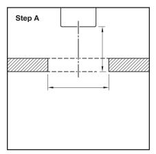
**Step A.** With reference to dimensions provided in Figure 8, install sprinkler fitting at proper distance above finished suspended ceiling level and cut clearance hole centered on sprinkler fitting through ceiling panel.
