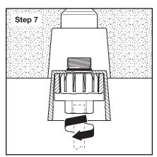
**Step 7.** Insert W-Type 28 Wrench (Figure 3) into installation cup cavity, fully seating and engaging internal cup ribs. Applying 27 mm hex wrench or 1/2 inch drive, unscrew Installation Cup from sprinkler fitting. Ensure O-ring is removed with Installation Cup from sprinkler fitting outlet and sprinkler cavity.
