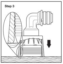
**Step 3.** Align Installation Cup with Cup Insert and press against concrete form. Ensure Installation Cup snaps into place, fully engaging Cup Insert, and is flush against concrete form.
