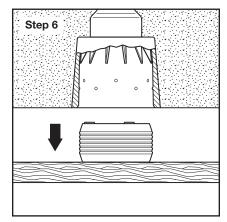
**Step 6.** After concrete has cured, remove concrete form with attached Cup Insert
