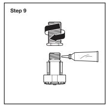
**Step 9.** Apply sealant to external threads of sprinkler inlet. With hex end of thread extension oriented toward sprinkler inlet, hand-tighten onto sprinkler threads until recess is seated on sprinkler thread shoulder.
