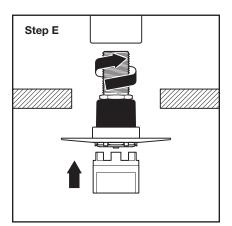
Step E. Engage Sprinkler by W-Type 25 Wrench (Figure 2). Hand-tighten (19 Nm [14 ft.- Ibs.] Maximum) assembly into sprinkler fitting. Ensure Escutcheon is flush against ceiling mounting surface and Sprinkler is oriented as intended (refer to Figures 1 and 2 for orientation details).
