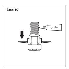
**Step 10.** Assemble Escutcheon onto sprinkler body. Ensure Escutcheon is flush against sprinkler body mating surface. Apply sealant to external threads of thread extension.
