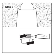
**Step 8.** Apply sealant (not included with sprinkler kit) to external threads of adapter. Hand-tighten Adapter into sprinkler fitting. Ensure adapter shoulder is flush against face of fitting.
