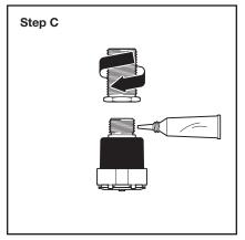
**Step C.** Apply sealant to external threads of sprinkler inlet. With hex end of thread extension oriented toward sprinkler inlet, hand-tighten onto sprinkler threads.
