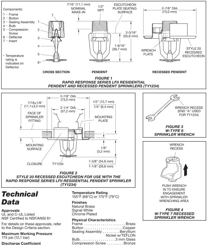
K=3.0 GPM/psi<sup>1/2</sup> (43,2 LPM/bar<sup>1/2</sup>)
