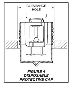
Do not attempt to compensate for insufficient adjustment in the Sprinkler by under- or over-tightening the Sprinkler/Support Cup Assembly. Re-adjust the position of the sprinkler fitting to suit.
