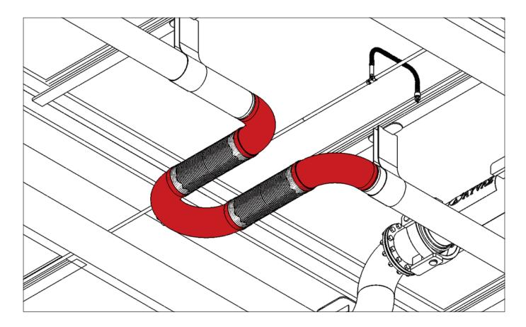
1. Ayvaz u-flex fire protection hose can be connected to pipeline with welding ends, flanges or grooved connection mounts through rigid or flexible couplings.
